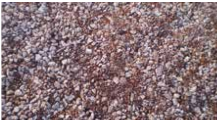
① DRAINING GROUND 10 - 15 cm Drainage layer formed by 10/15 cm of volcanic lapillus, grain size 5-20 mm, crush resistance 35 N/mm 2 (UNI 7549/7).
